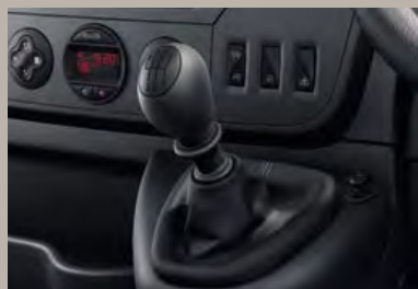
Six-speed manual gearbox
