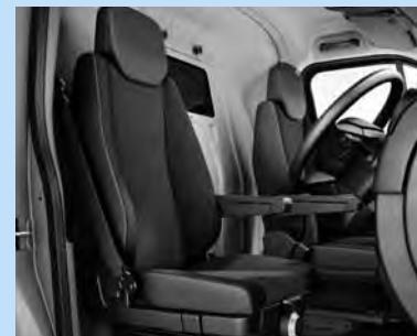
Air-suspended driver's seat with armrest.
