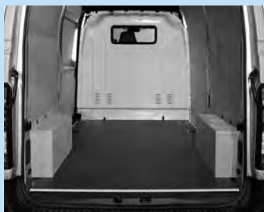
Full-height plywood load lining panels and wheel arch protection.
