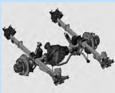
Rear axle: Rear-wheel drive.
