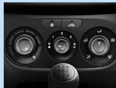
Air conditioning and air recirculation.
