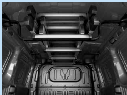
Internal ladder storage bars.
