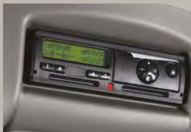
Optional digital tachograph** Computes driving and rest time, enabling fleet management data to be analysed.
