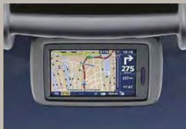
Satellite navigation The optional TomTom based unit includes hand-held/facia-mounted remote control.
