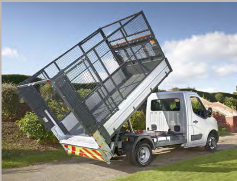
Movano L2 H1 R3500HD chassis cab fitted with the VFS Caged Tipper. 500kg 'dump-over' tail lift with 765mm deep folding aluminium platform is optional at extra cost.
