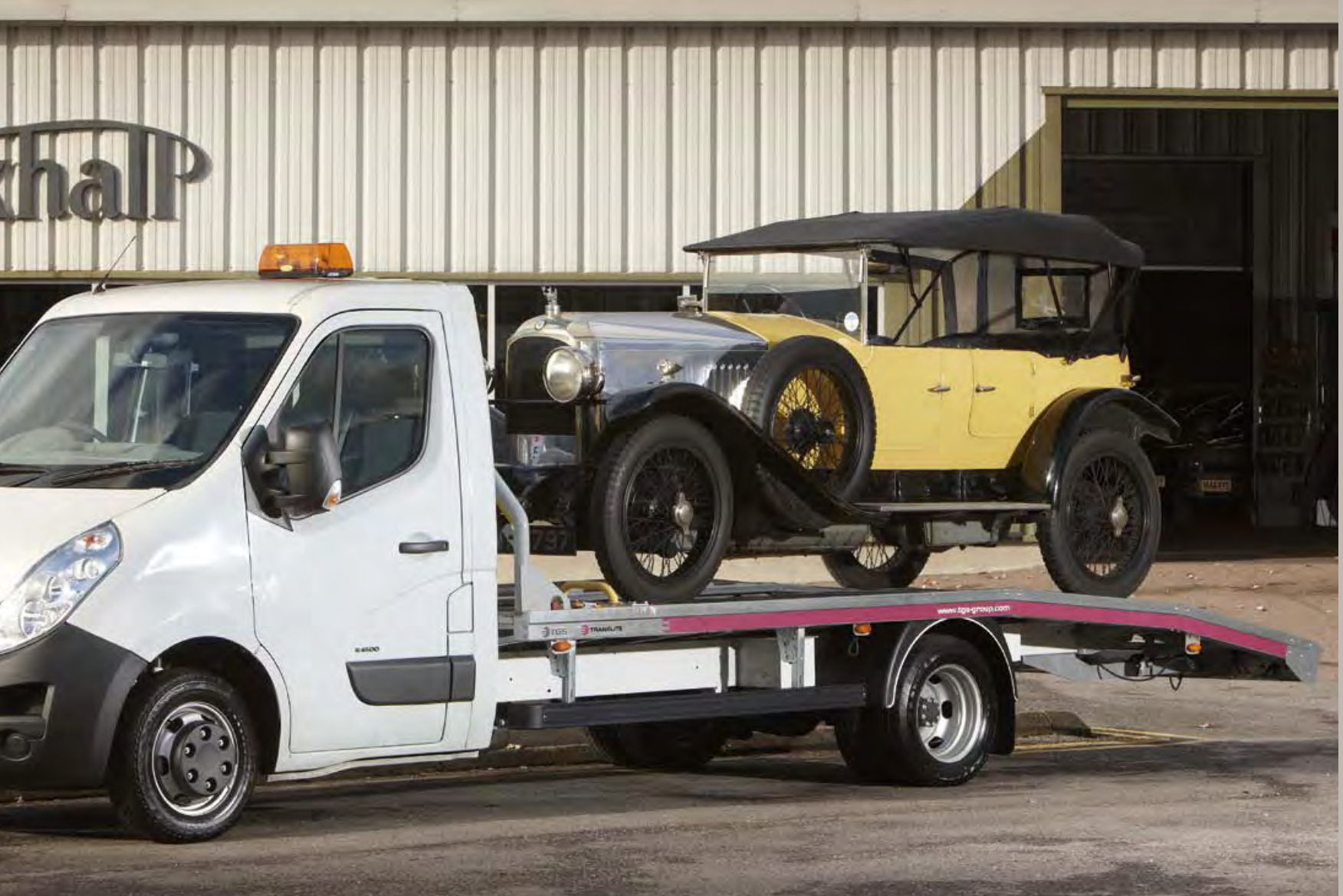
Movano L4 H1R4500HD Chassis Cab featuring the Translite Car Transporter conversion.
