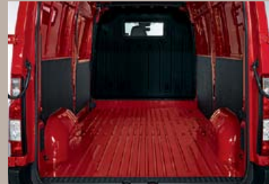
Load area protective panels Half-height load trim panels help safeguard the side walls from everyday wear and tear. Standard on RWD models.
