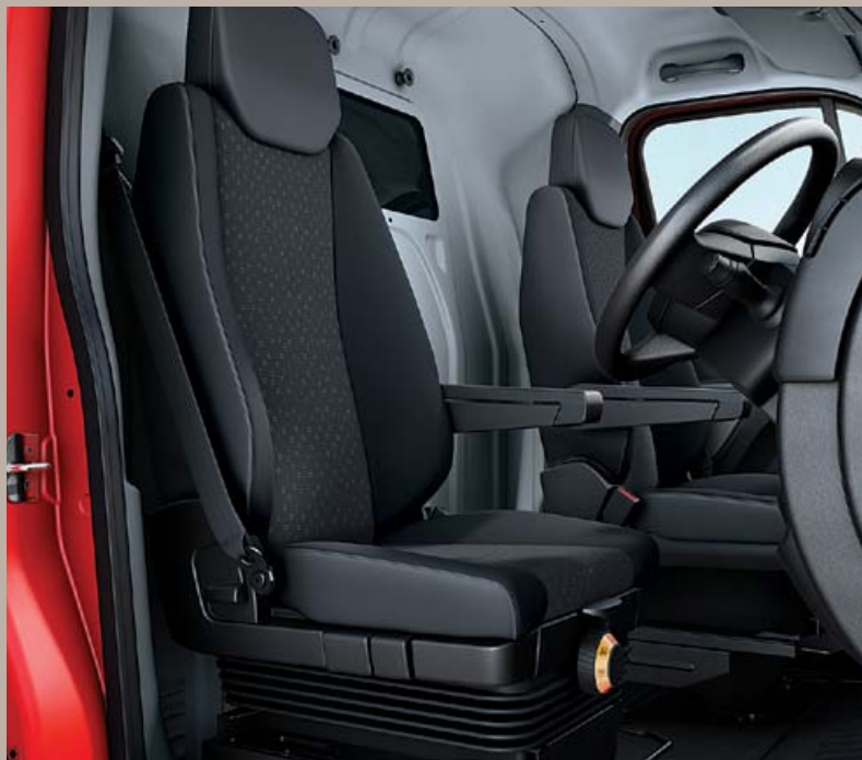
Air-suspended driver's seat The eight-way adjustable, air-suspended driver's seat features an armrest and adjustable suspension sensitivity for maximum comfort in all conditions.
