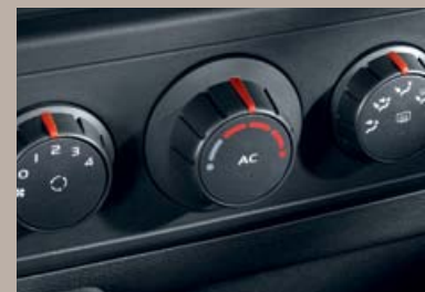
Air conditioning Comes complete with pollen filter and chilled glovebox. Aids demisting and provides a fresher travelling environment all year round.
