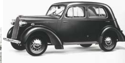
1937 – The Vauxhall 10' H-type, the first British car to have integral construction.
