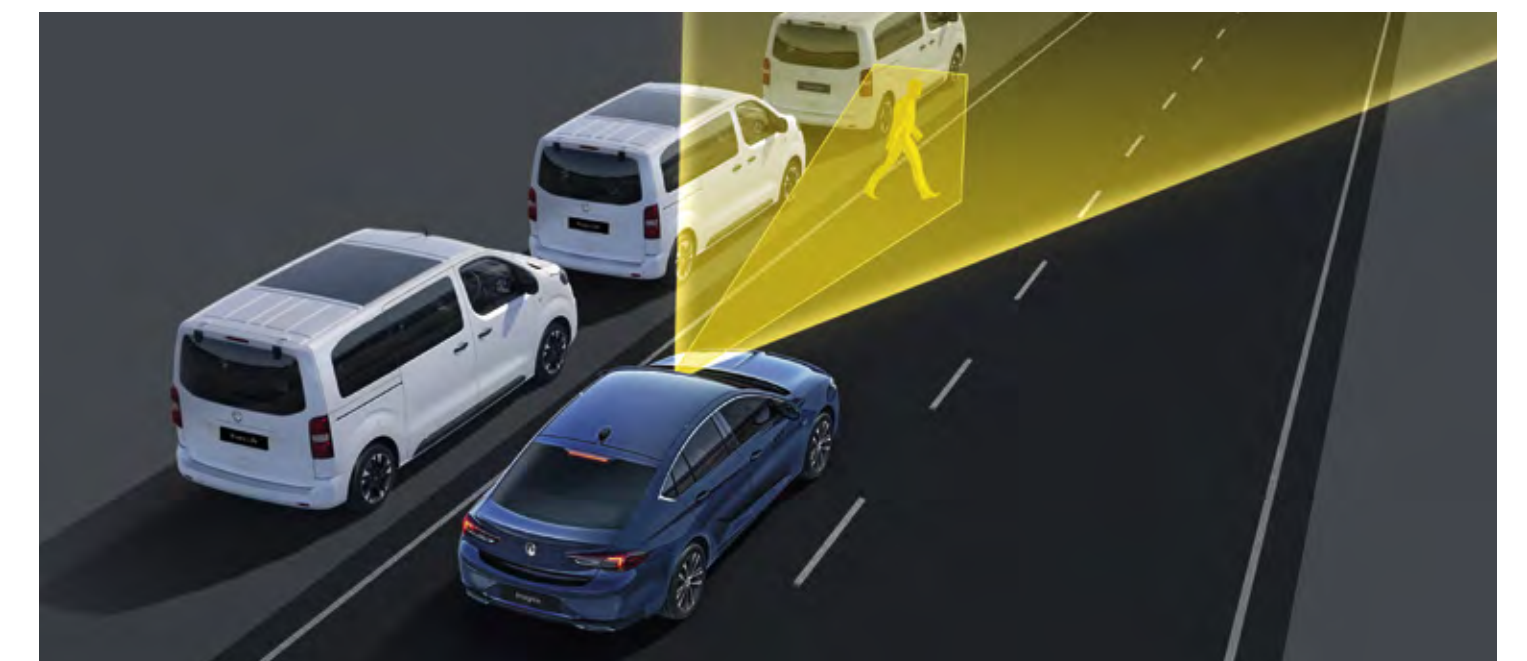
Automatic emergency braking with pedestrian detection.
