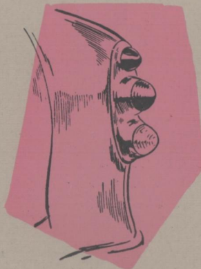
GROUPED TAIL, STOP AND REVERSING LAMPS
