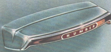
Petrol Filler Hinged panel in rear wing conceals petrol filler cap: neat, accessible.
