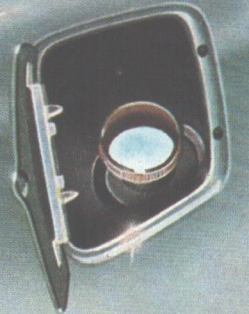
Petrol Filler Hinged panel in rear wing conceals petrol filler cap: neat, accessible.
