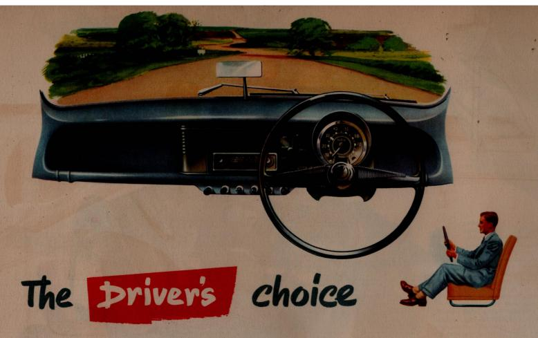
The instruments which include speedometer, fuel gauge, ignition and oil pressure warning lights are neatly grouped in full vision of the driver and are hooded to prevent reflection on the screen.
