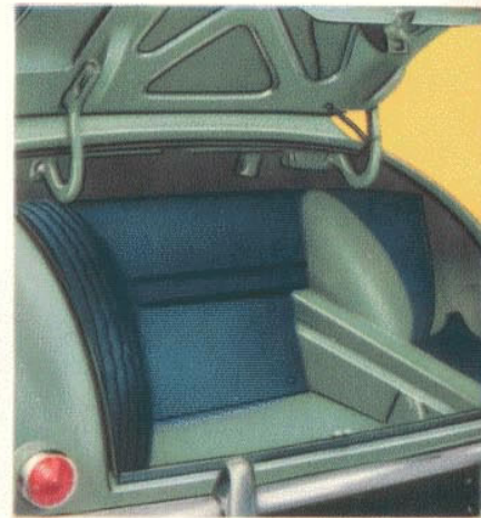
This capacious boot provides all the luggage space you need. For effortless opening, the lid is counterbalanced with torsion bar hinges.
