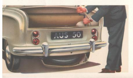
The spare wheel is carried unobtrusively beneath the luggage compartment on a separate tray. This is lowered close to the ground by means of the starting handle and raised again just as easily by the same method.
