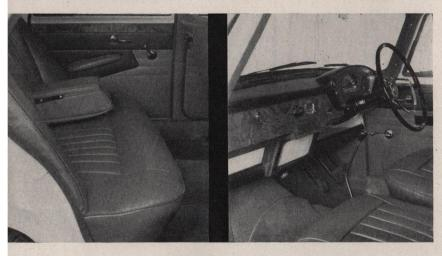
Front seats are of the fully adjusting bucket type. Rear seat has fold-back central arm-rest and door-pull side-rests.
