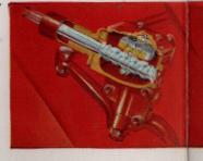
A high-efficiency steering unit of recirculating ball design gives precision control – makes handling easy under all road conditions.
