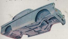
The Sunbeam Rapier has all-steel unitary construction, the strongest and safest form of body-chassis structure.
