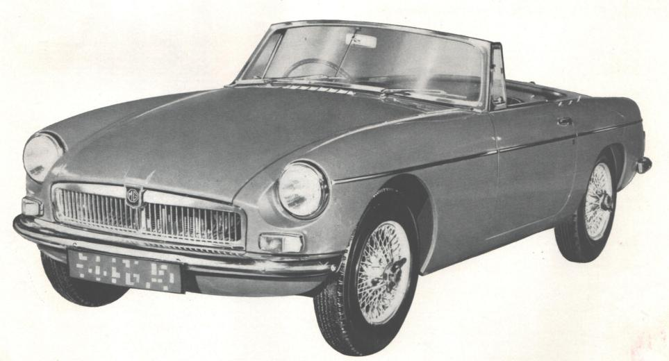
The bonnet lid is of aluminium for lightness, while the windshield frame is of polished aluminium to avoid rust. Wrap-round bumpers with over-riders front and rear (optional on front for Home market), double-dip, sealed-beam headlamps, a heater air intake on the bonnet top clear of exhaust fumes, and a rear-view mirror adjustable for height are examples of some of the many worthwhile features of the 'MGB'. A wide range of optional extras is offered, including the wire-spoke wheels illustrated.
