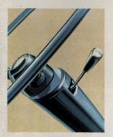
A single switch on the steeringcolumn incorporates dip switch, headlamp flasher, horn, and selfcancelling direction indicators; thus providing a single source of all communications with other road users.
