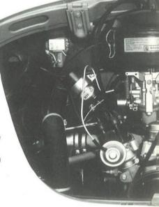
4 cylinder, horizo opposed rear mocooled. Output SAE 60 b
