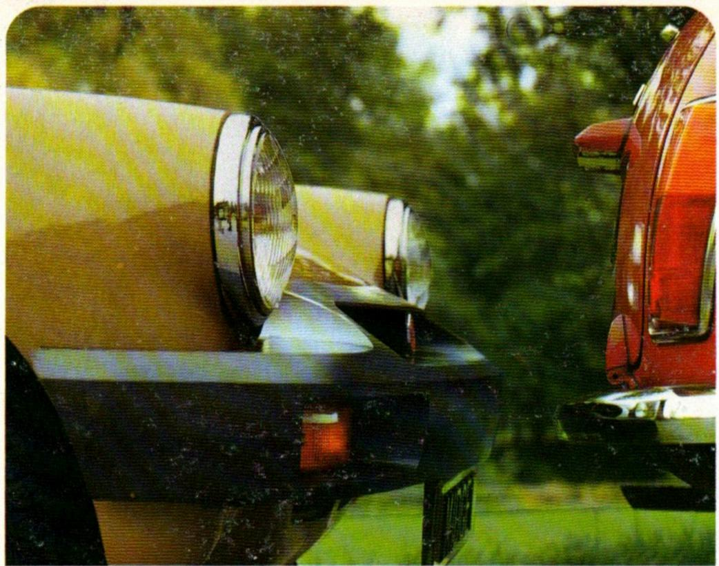
Those full-width polyurethane bumpers have a more important b to do than merely bolstering the Midget's appearance -although they do that handsomely! They're designed to foil the car-park 'nudger' by soaking up low-speed impact, so helping your Midget to keep its good looks.
