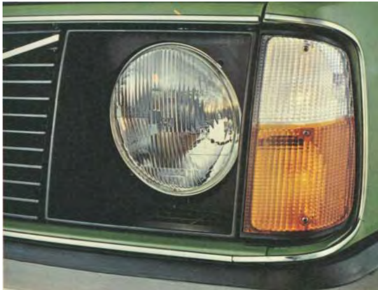
The halogen headlights are bigger this year -180 mm in diameter - for safer night driving. The main beam is longer and the dipped beam is wider, both are more intensive.
