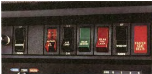
These are the controls for the electrically-operated windows and air conditioning in the Volvo 264 GL. Also shown are the switches for the electrically
