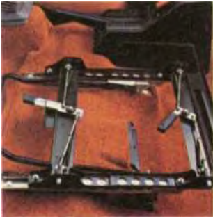
Driving seat height can be adjusted quickly and simply by means of two levers, one for the front of the seat, one for the rear.
