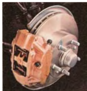
The Volvo 264 has power-assisted disc brakes all round. Relief valves in the rear brake lines prevent premature lock-up of the rear wheels in emergency situations.
