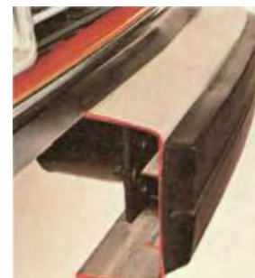
These very strong shock absorbers protect the car body from damage at speeds up to 5 km/h. Which could save a lot of embarrassment, not to mention repairs.
