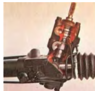
The new power-assisted rack and pinion steering, as well as making light work of city driving and parking, improves directional stability and steering response.
