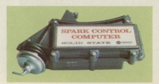
The brain of the Lean-Burn System is this electronic spark-control computer which responds to data from 8 sensors and instantly adjusts the timing of spark-plug firings to achieve the best combustion efficiency for all conditions. Since conditions are constantly changing, the computer is constantly making instantaneous adjustments in spark-plug firings. This results in good engine performance.
