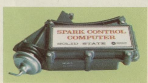
The brain of the Lean-Burn System is this electronic spark-control computer which responds to data from 8 sensors and instantly adjusts the timing of spark-plug firings to achieve the best combustion efficiency for all conditions. Since conditions are constantly changing, the computer is constantly making instantaneous adjustments in spark-plug firings. This results in good engine performance.
