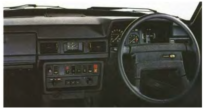
The instrumentation includes a comprehensive system of warning and reminder lights.
