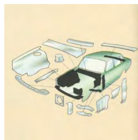
The resistance to rust of a Volvo 264 is built in from the start. Exposed body sections are galvanised. Totally, each car of the 260 Series uses not less than 3.5 square metres of galvanised sheet steel.
