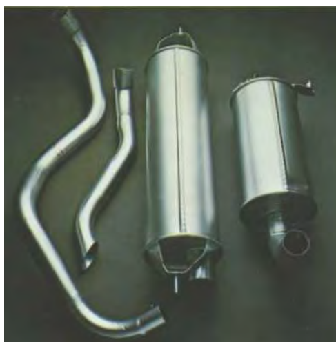
The vulnerable, exposed parts of the exhaust system are aluminised.
