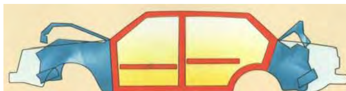
The Volvo 264 is strong with built-in weaknesses! The front and rear sections of the body are designed to act as crumple zones, soaking up the impact of a crash. The occupant area is protected by an extremely strong framework of steel profiles and tubular members.
