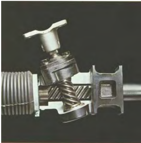
Feel the directional stability and exactness of rack and pinion steering.
