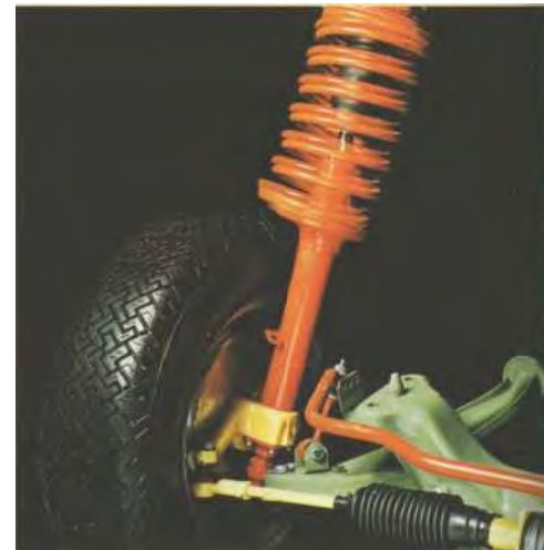
The Volvo 264 has a front suspension of spring strut type which takes the bumps in its stride for a smoother, better ride.
