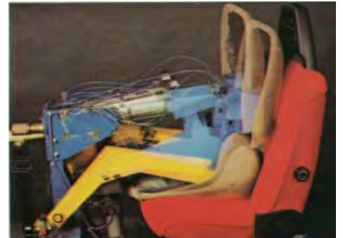
Durability tests are carried out on all important components before they can be said to meet the 'Volvo' standard of quality.
