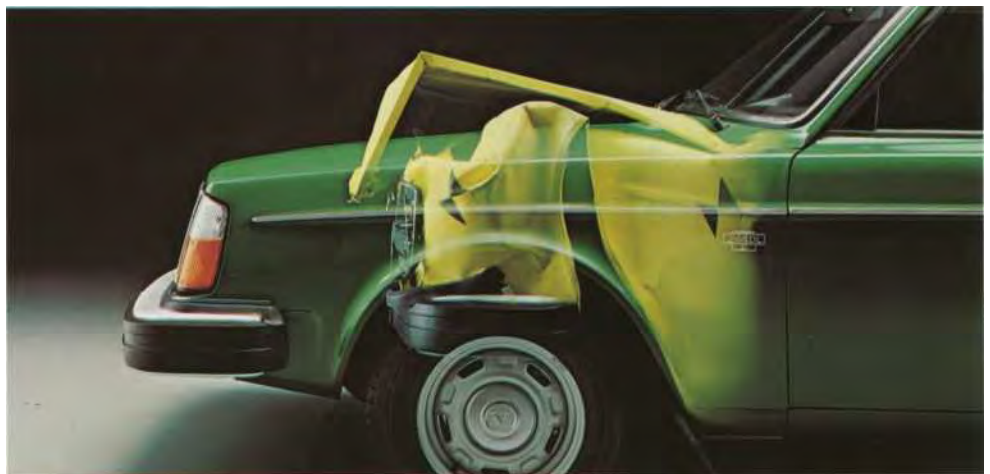
The front end absorbs the impact of a collision. Thus it decreases the risk of serious injuries.
