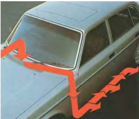
Slipstream air ventilates door sills to prevent moisture and corrosion.
