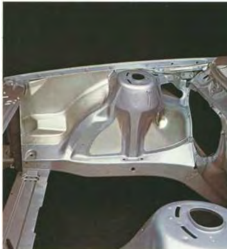
Generous use of highly corrosion-resistant double-sided hot zinc plate (zinc layer 3-4 times the thickness of most other car makes).
