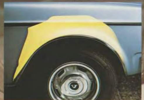
The front wheel housings have separate protective inner mudguards made of polypropylene to protect the body against flying gravel and dirt deposits. This also reduces the risk of corrosion.
