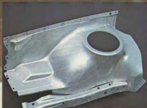
All exposed body parts are made of zinc coated sheet steel to minimise corrosion.
