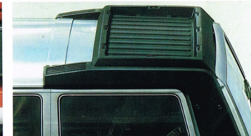
Fresh-air intake opening with additional roof-mounted luggage tray.
