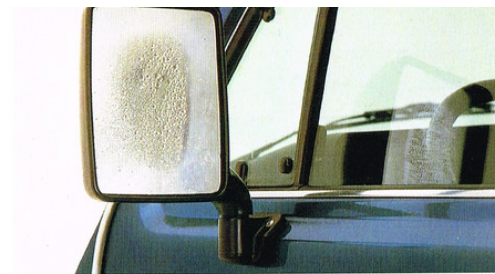
Electrically heated, remote-control door mirror.
