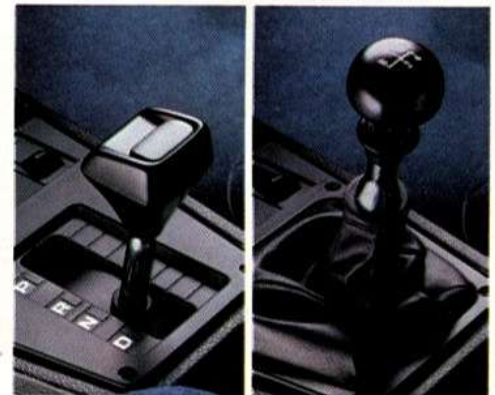
Automatic transmission lever has four positions: D (forward drive), N (neutral), R (reverse drive) and P (parked position).
