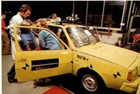
Crash testing involves the use of specially designed dummies. They are placed in the car and connected to sensitive instruments which accurately record all reactions caused by the crash.
