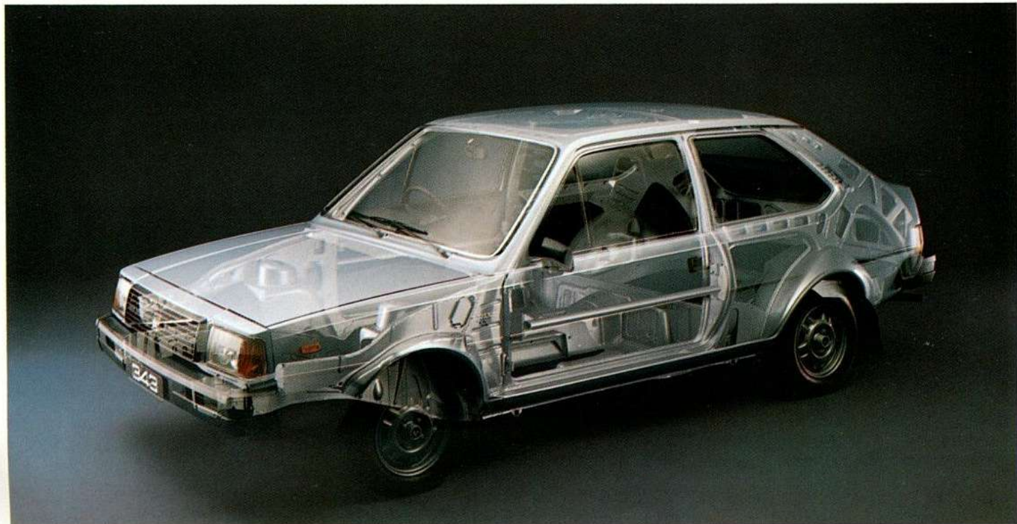
The safety-type steering column, fitted with a firm padded safety-type steering wheel, gives way in head-on collisions. This protects the driver from injury caused by the steering column being forced back inside the car.
