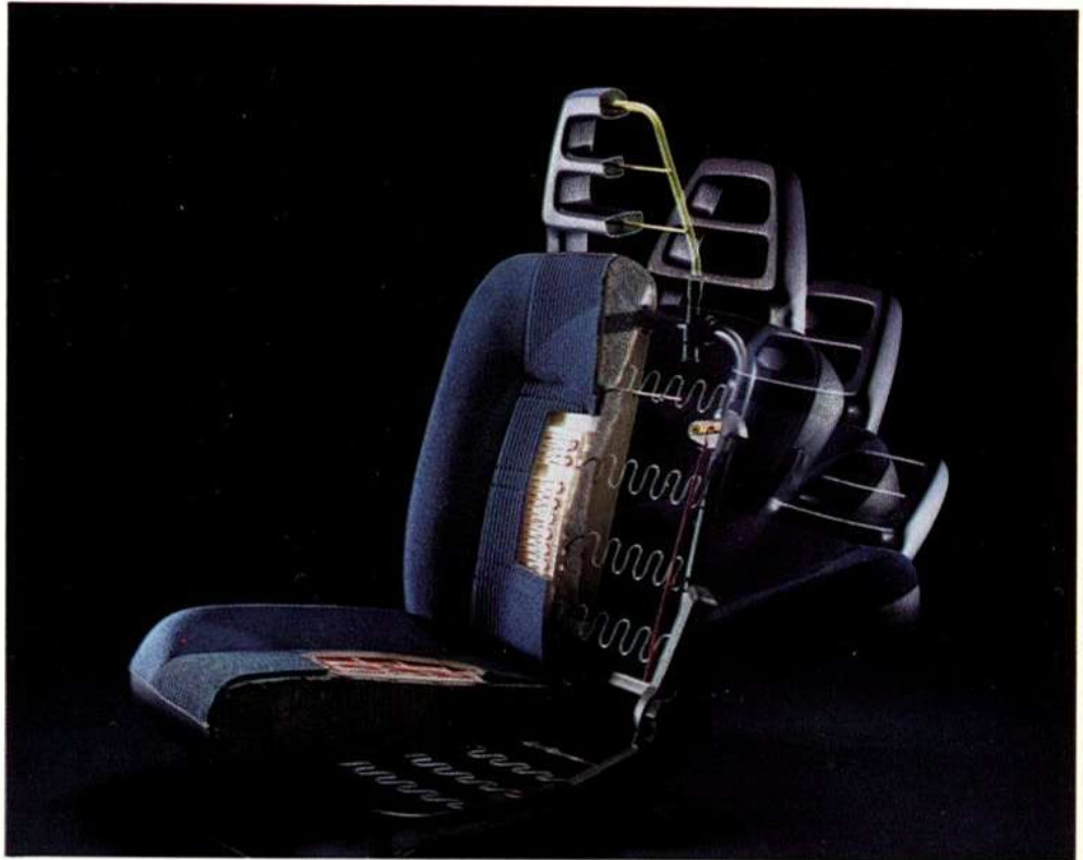
The seat backrests can be adjusted to the fully reclined position, and the front seats can be moved on the runners over a distance of 10 inches.
