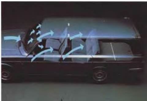
1. 14 inlets make for an abundant availability of ventilation.
