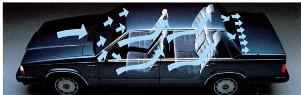
13-outlet heating and ventilation system
