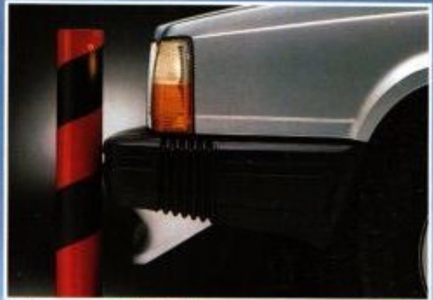
The bumpers can absorb collisions at speeds of up to 4km/h
