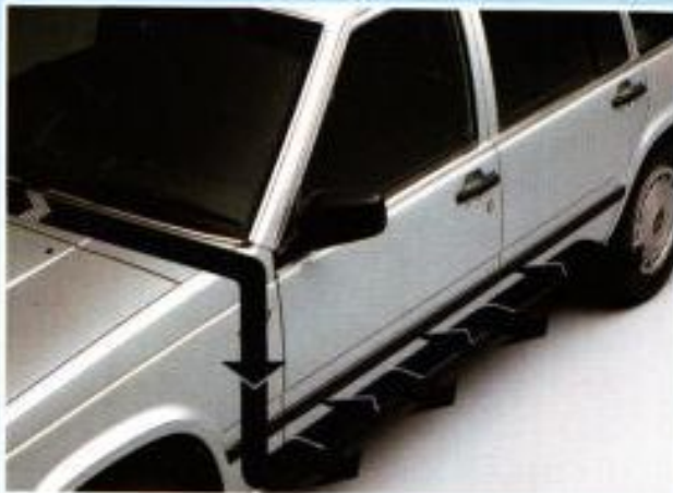
Ventilated door sills for lasting protection
