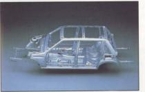
Crumple zones and a rigid steel cage combine to provide maximum protection for passengers.
