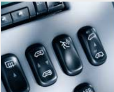
Anti-theft alarm system with tow-away protection sensor (battery horn can also be included)
