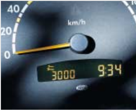
"Assyst" service interval indicator for flexible oil service intervals
