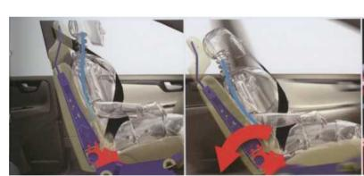
WHIPS (Whiplash Protection System) reduces the strain on the spine and neck in rear-end collisions. It is integrated in the front seats and is activated if a rear impact is sufficiently severe.
