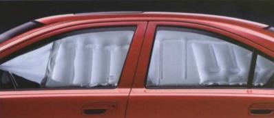
Volvo's unique SIPS side-impact protection system uses a large part of the car body to absorb the force of an impact. The IC (inflatable curtain) and side airbags provide maximum protection for the head and chest in a side impact.
