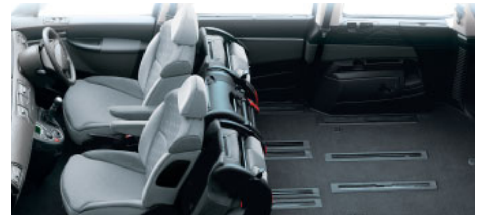
Putting seats in the "wallet" the position frees up maximum boot space.
