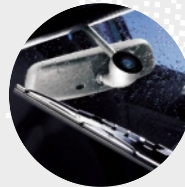
A rain sensor regulates the speed of the wipers depending on the weather conditions.
