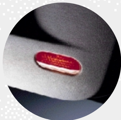
At night-time, the door-mounted 'puddle' lights illuminate the ground when opening the front doors.
