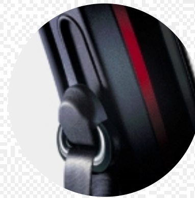
For greater comfort and safety, the front seat belts are height-adjustable.
