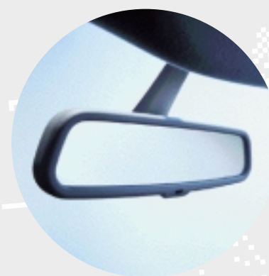
The automatic dimming interior rear-view mirror darkens if a following car's lights are too high.
