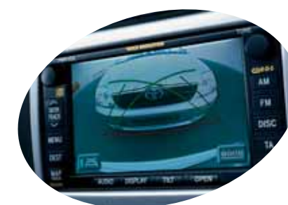
The optional rear view monitor system offers a valuable aid to reversing. Once reverse gear is engaged, a wide-angle TV camera on the back door transmits the rearward view to the multi-display screen in front of the driver.
