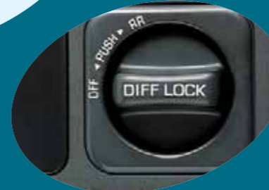
The rear differential lock provides power to where it's most needed in extreme off-road conditions (diesel only).
