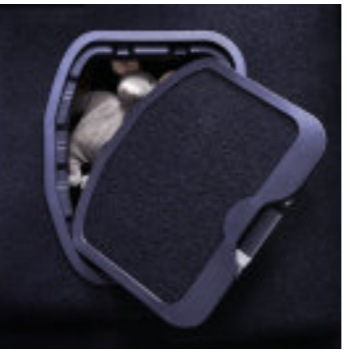
9. Rear foot wells incorporating two secret stow-away compartments with lids (one only when JBL is fitted).
