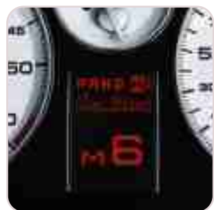
The gear selected is shown on the instrument panel.
