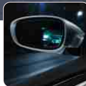
Electrochrome rear-view mirror stops you being dazzled from behind.
