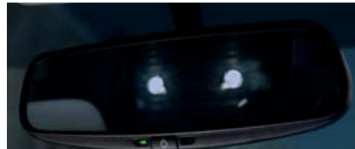
The electrochromic rear-view mirror cuts glare by automatically dimming the headlight reflection from following cars.
