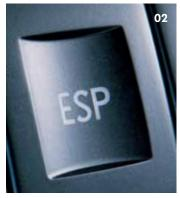
Programme - ESP - helps to prevent losing control in unstable driving conditions.
