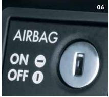
**06** The front passenger airbag can be deactivated, to allow the use of a rear facing child seat, by the simple turn of a key.
