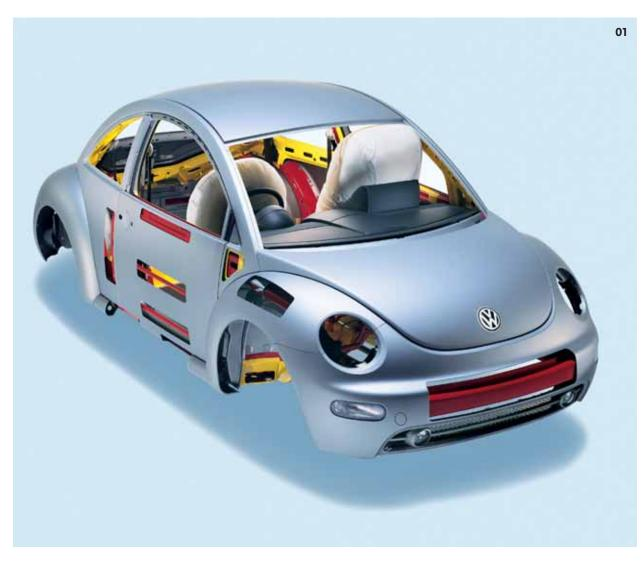
**01** Front and rear crumple zones and a reinforced inner safety cell help protect you and your passengers in the event of an accident.
