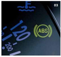
**02** The Electronic Stabilisation **03** ABS helps you to steer around potential hazards, under hard braking, by preventing the wheels from locking.
