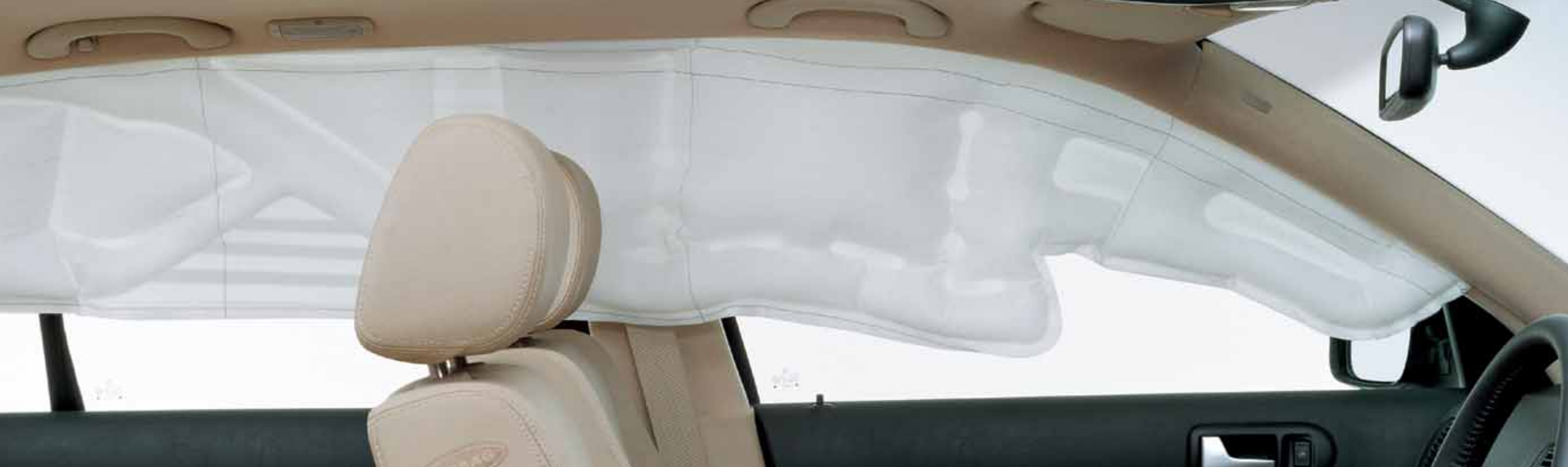
The curtain airbag system is available as an option on all models.
