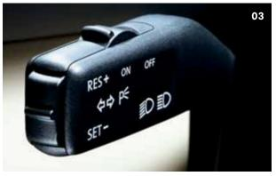
**03** On long journeys, cruise control is a real bonus. It can maintain a constant speed from 20 mph upwards and automatically switches off when the brake or clutch is engaged.
