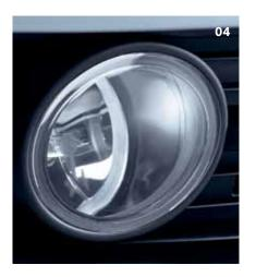
**04** Front fog lights integrated in the front bumper provide both safety and aesthetic appeal.
