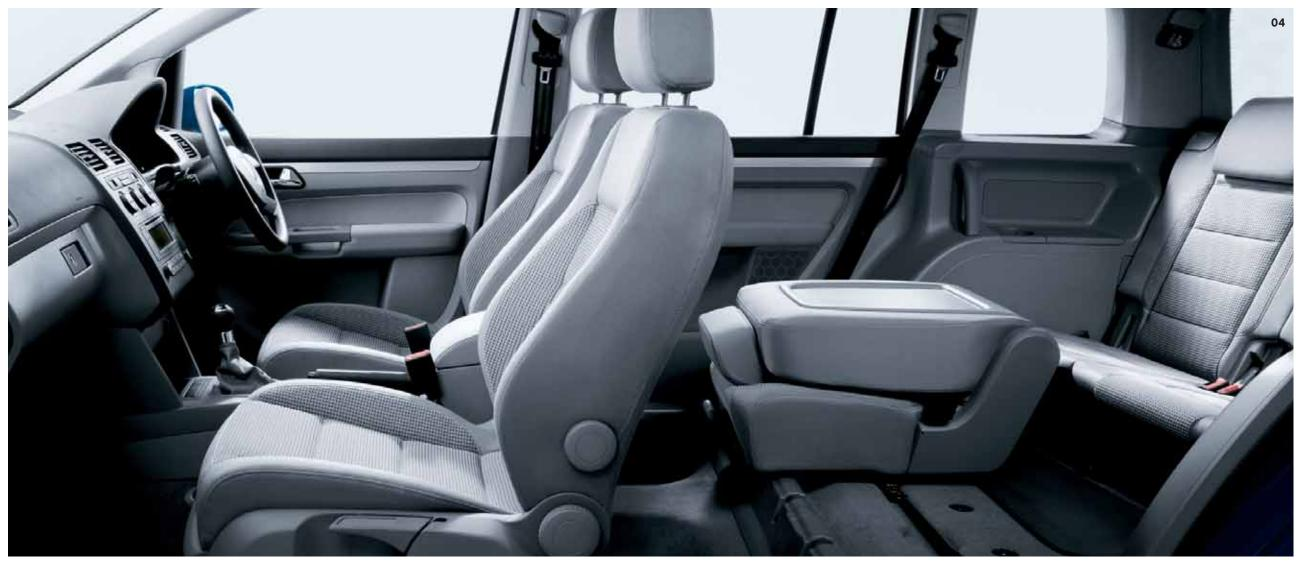
**04** With the two outer seats of the second row removed, there's ample room around the middle seat that converts into a table. Interior shown is Sport.
