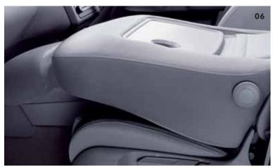
**06** The front passenger seat can be folded flat to transform into a handy table.
