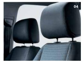
04 The driver and front passenger benefit from active head restraints which help lower the risk of whiplash injuries in the event of an accident. In addition, side airbags provide greater protection for the driver and front passenger, whilst the curtain airbag system protects the front and second row passengers.
