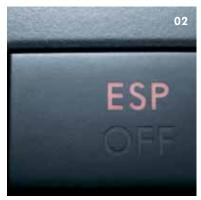
**02** The Electronic Stabilisation Programme (ESP) detects critical situations at an early stage and takes action by, for example, specifically braking individual wheels.
