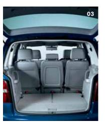
o3 The single seats of the second row, each weigh less than 16 kg allowing a fast and easy choice between seating and luggage space.
