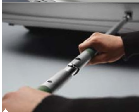
Safety tow rod 2-piece steel rod with patented connector and cotter pin. For trailer couplings and towing eyes. Approved for vehicles with a gross vehicle weight of up to 3.2 t
