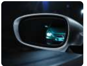
The electrochrome rear-view mirrors prevent you from being dazzled by the headlamps of following vehicles.
