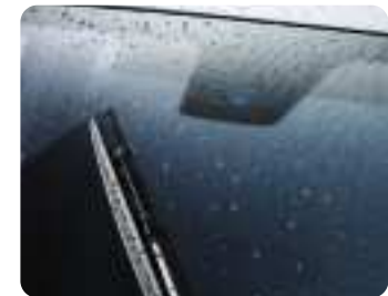
The rain sensor activates the windscreen wipers as soon as it starts to rain.
