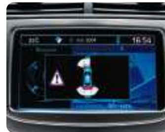
Parking assistance is also displayed in the form of graphic bars on the multifunction display.
