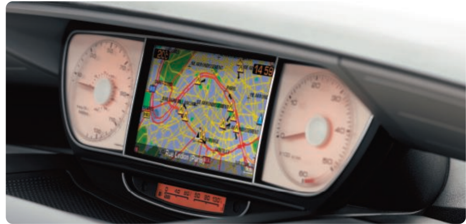
Directions can be read directly from the large colour screen situated on the RT3's instrument panel, with its off-white background and orange lights.
