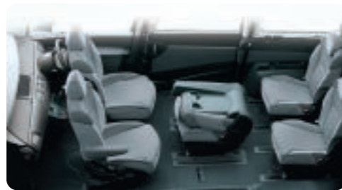
Park and take it easy. In the 'lounge' (1) configuration you can swivel the front seats round and fold a centre seat down to form a practical low table.
