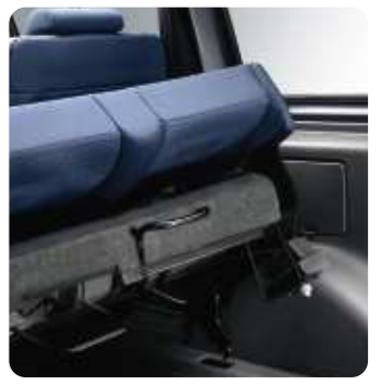
The practical seat fixtures of the Expert Combi make it easy to install and remove the 3-seater bench seats, which can be done in three quick steps. (2 people are needed for this operation).
