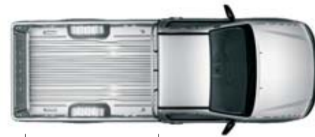
Hilux Single Cab has a deck width of 1520 mm, deck length of 2315 mm and deck height of 450 mm.
