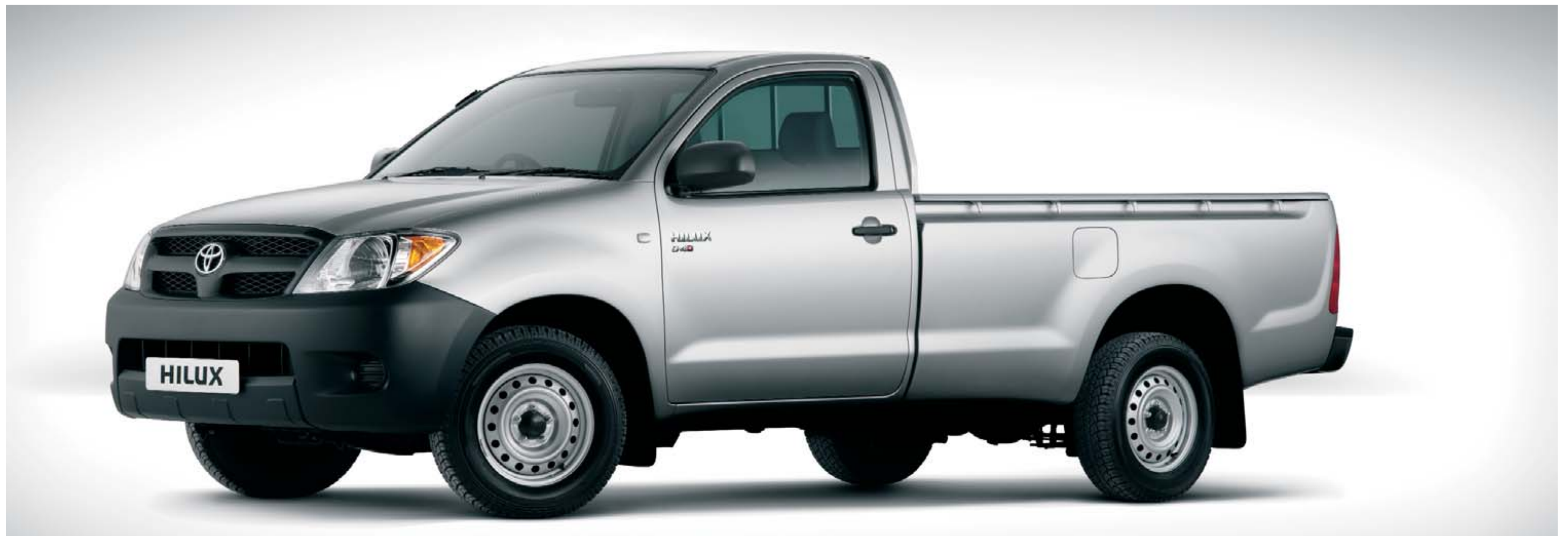
Hilux Single Cab has a deck width of 1520 mm, deck length of 2315 mm and deck height of 450 mm.
